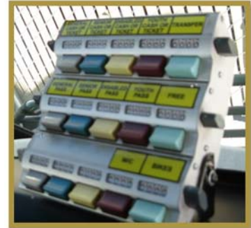
Figure 4-8: Passenger Counter on Yuba-Sutter Transit Fixed Route Vehicles
